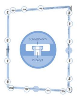
Turn-tilt windows made of wood and PVC-U now achieve a high level of RC3 burglary resistance with standard components from the Winkhaus activPilot fitting system. Its all-round fitting linkage with evenly arranged locking points offers a high level of security and ease of use. And the hardened drilling protection and airgap limiters, which are adapted to the installation situation, ensure a high level of resistance even during attempts to lever the window open with heavy tools.
